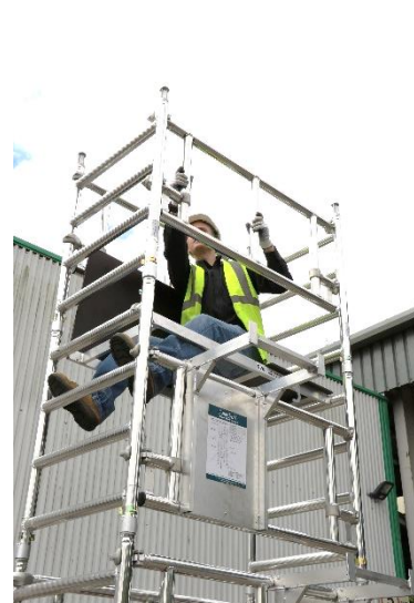
28. Fit 2 guardrail frames, with the top hook (facing outwards) set above the top rung of the frame.
