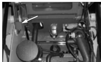
Figure 24 ROPS Lock Mechanism
