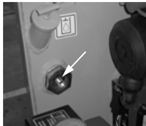
Figure 30 Hydraulic Oil Service
