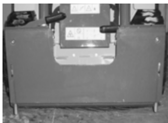
Figure 13 All-Tach® Bracket Mechanism (Hitch)
